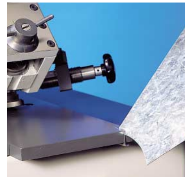
Pre-bending a flange with an adjustable stop as feeding support.
