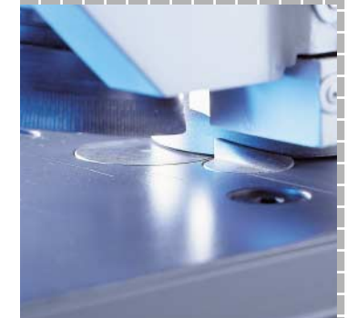
Hardened sliding nose and pressure plate for plasma cut blanks.
