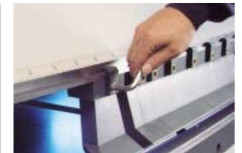
With the quick clamp system, tools can be changed in seconds. The tool seat is integrated directly into the upper beam.
