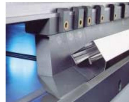
The boundless front and side free space can accommodate return flanges up to 56 mm (2.165").
