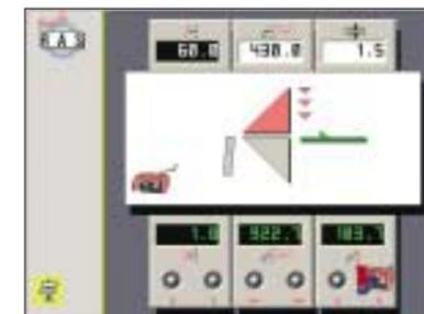
If someone operates the machine occasionally, he can use the EasyGo operation. Simply enter an angle, a backstop dimension and the material thickness and you are ready to go. If you want to bend "by eye" just press the push buttons and start each machine movement separately.
